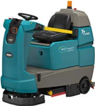
Tennant's T7AMR Autonomous Mobile Robot
